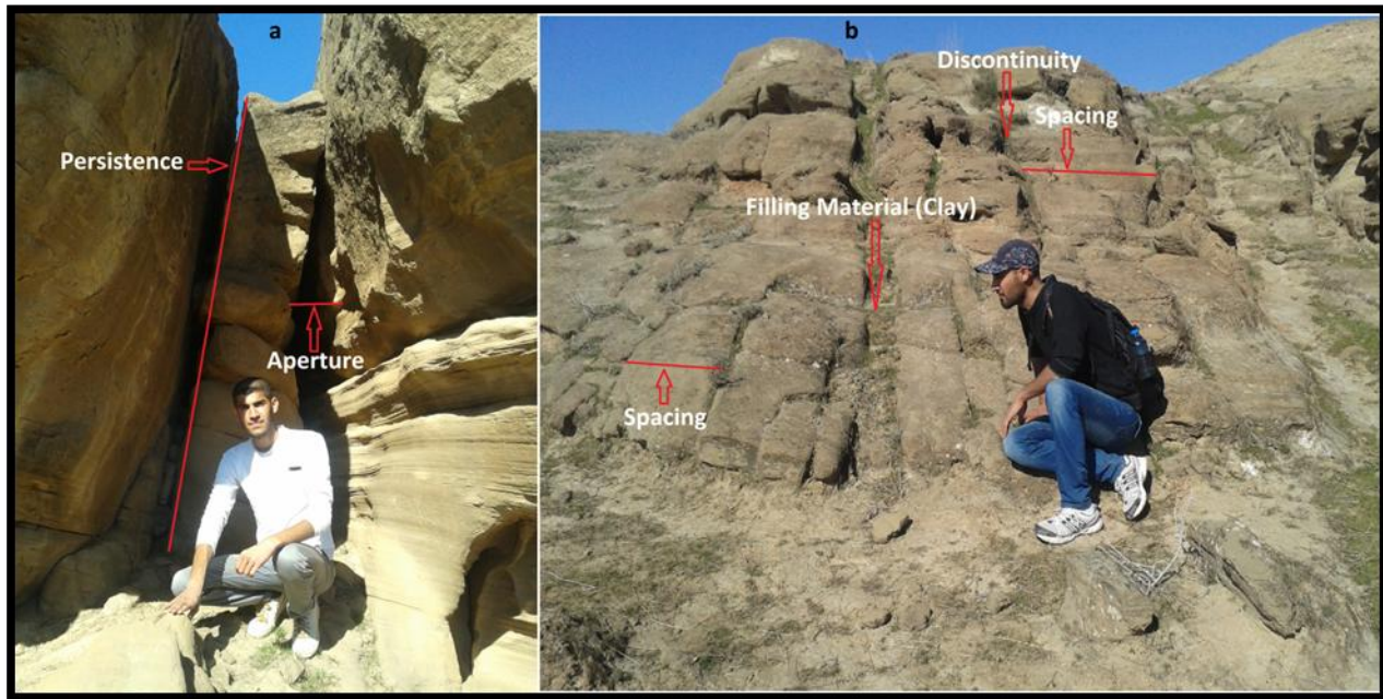
Fig.6 a) shows persistence and aperture, b) shows filling material and spacing of discontinuities in the study area
